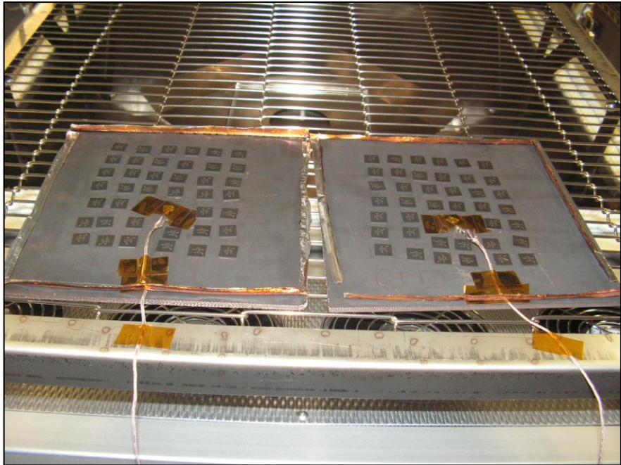
Figure 1: SMDs positioned on carriers inside the reflow oven
